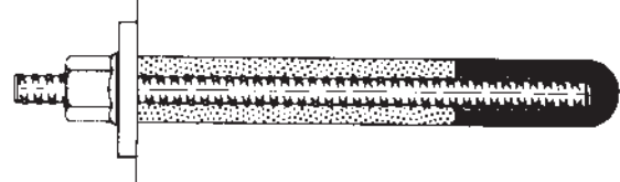
Tensioned bolts fully resin anchored and grouted.
