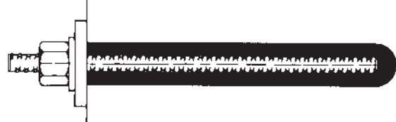
Untensioned dowels fully resin grouted.
